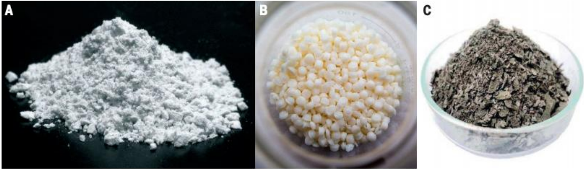
Struvite (A), polyhydroxyalkanoate bioplastic (B), and alginate biopolymers (C) are examples of recycled materials produced by wastewater treatment.
